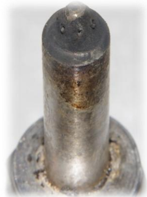
Contaminated fuel injector
